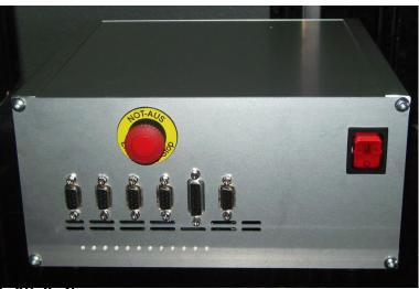
Motor connectors (X1, X2, Y, Z)
